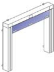
F. Touch and hold velcro drop curtain (12"-18" drop).
