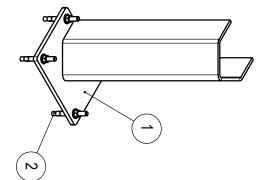
NOTE: ANCHORS NOT INCLUDED MATERIAL: %" STEEL, %" BASE PLATE, POWDER COATED YELLOW
