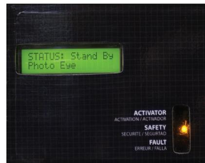
(FIG.3) YELLOW LED LIGHT IS ON WHEN REVERSING DEVICE HAS BEEN ACTIVATED OR TRIPPED
