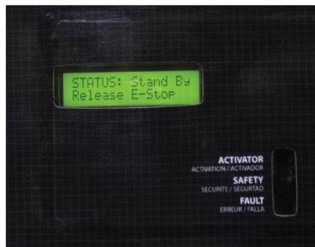
**(FIG.7) E-STOP = EMERGENCY STOP ACTIVATED**
