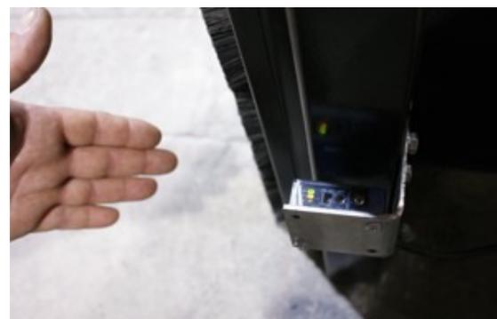
(FIG.5) **NOTE:** GREEN and YELLOW LED's are “ON”, an object in way of beam thus correctly tripping the activation or reversing feature.
