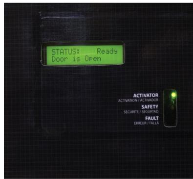
(FIG.2) GREEN LED IS 'ON' WHEN ACTIVATOR DEVICES ARE ACTIVATED OR IF WIRING INPUT PROBLEM
